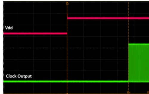
Figure 16. Startup Waveform vs. Vdd
